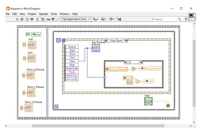
The three variables, "Num\_q\_Presses", "Num\_r\_Presses", and "Num\_3\_Presses" are not needed in your code. These variables are just incremented by one each time the Key Down event is called and that specific key was pressed.
