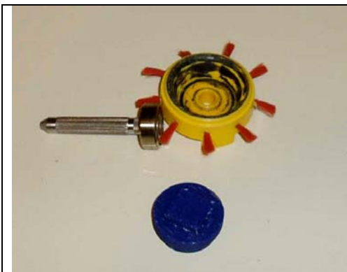
The part – in blue – now cleaned of the support material
