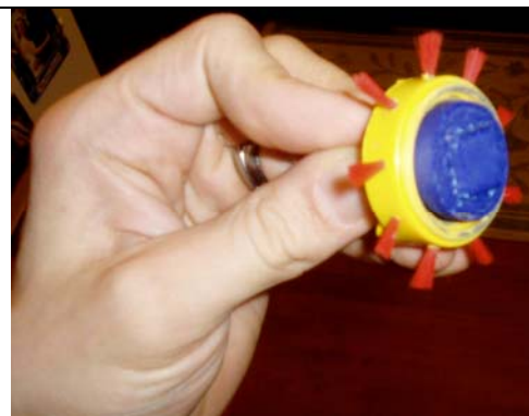
The part (installed) is a bearing mount
